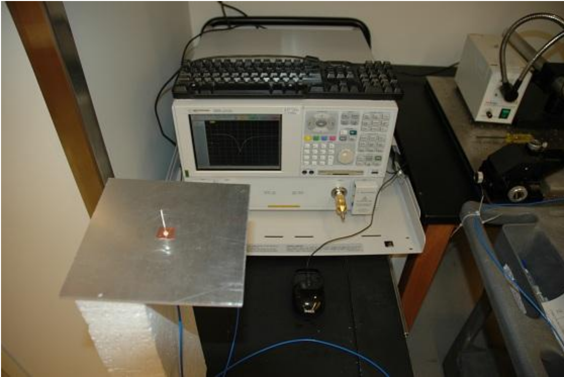
Fabricated monopole, and measurement setup (with permission from CMIP, Duke University)
